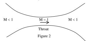
**10.1.** Maximum Mass Flow Through a Nozzle. We consider a channel which is tapering steadily to a minimum section at the outlet. Let A be the section at the outlet of the channel where the velocity is u, pressure p and density  $\rho$ . Then, applying Bernoulli's equation along a stream-line from the reservoir to the section A, we get
